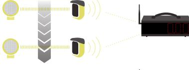
• in combination with the Witty•TIMER; pulses transmitted by the photocells are received by the board and by the timer independently, but in this case, with the timer function, data can be saved and stored for analysis subsequently on a computer using the Witty•MANAGER software package
